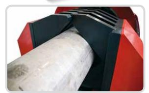
Semi-automatic unit structurally strong and at the same time user friendly. The locking vice design enables the automatic centring and positioning without causing deformation to the pipe.
