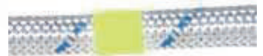
Luminous strip aids the operator to centre system to the weld gap
