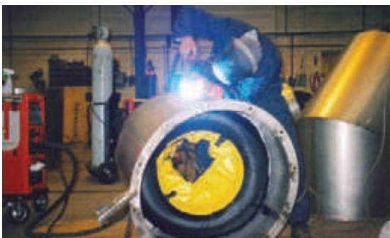
Speedy Purge used to weld a stainless steel elbow.
