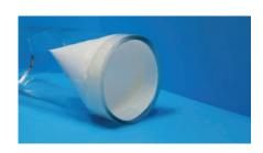
WS Purge Dams are preformed water soluble purge dams. These preformed dams are size specific and each cone can be used on all wall thicknesses and pipe schedules. Each pack includes 2 pcs of 'Fixing Tape' and the required length of water soluble tape. They will completely dissolve without any risk of residue. Available in all sizes from 2" to 36". Sold individually.
