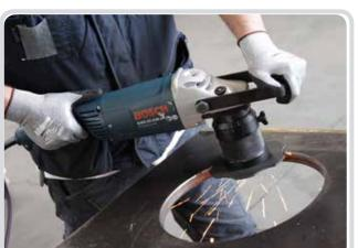
Also available are a milling head and inserts for radiusing sharp edges (R3, R4, R5).
