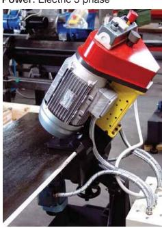
The **Edge 46** produces bevels using an insert-type high speed milling head, enabling a high material removal rate, while keeping replacement consumable costs to a minimum. Bevelling tips have 4 cutting edges and are available to machine all types of material.
