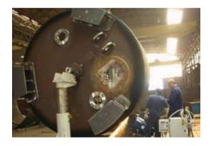
GBC G400 shown mounted on trolley, during typical back gouging operation, circumferential on O.D. of pressure vessel. The trolley allows easy handling and moving of the grinding head.
