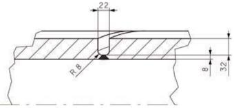
Example with ferrule diam. 2000mm wall thickness 40mm material A516 Gr. 70.
