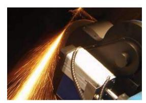
G 400 Grinder pneumatic feeding system compensator retracts the feeding piston when it encounters ovality to eliminate excessive material removal.
