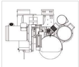
Grinding head can turn of 90° for dedicated set up when performing longitudinal back gouging (mounted on column welding boom arm only).
