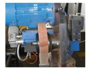
Optional flap wheels for polishing, cleaning and removal or reduction of weld seam.
