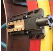
The unit is also equipped with two copier toolboxes with the spring loaded pipe OD tracking system, minimizing the bevel offset on out of round pipe.
