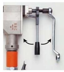
Lever handle for feeding the cutter head in tight spots where manual feeding is impossible.
