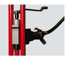
Pipe beveler MINI C40, pneumatic version, with 40mm body and cutter head for jobs in extremely restricted access areas. RANGE: 20-39 mm I/D (optional from 12,5 mm)
