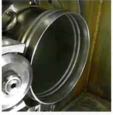
Achieves a burr-free cut once the cut has been completed, allowing the operators to handle the opened container without chance of cuts to gloves or hands.
