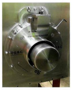
Hermetically sealed design allows for the SL160 to be mounted to glove boxes and other containment vessels with confidence - all machines are supplied vacuum tested to 0.05% leak rate prior to signing off of LTQR's
