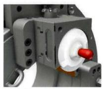
Quick change tool cartridge with magnetic guarding protects the operator from sharp edge of the cutting wheel and offers ease of replacement when worn
