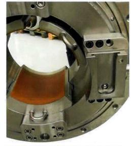
Size specific, quick change clamping pads give full support to the can OD ensuring accurate centring for effective repeatable cutting results
